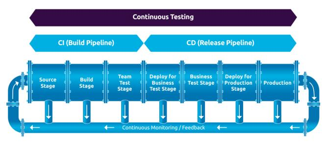
Figure: Basic setup of a CI/CD pipeline (Figure 6.1 of the book Quality for DevOps teams)
